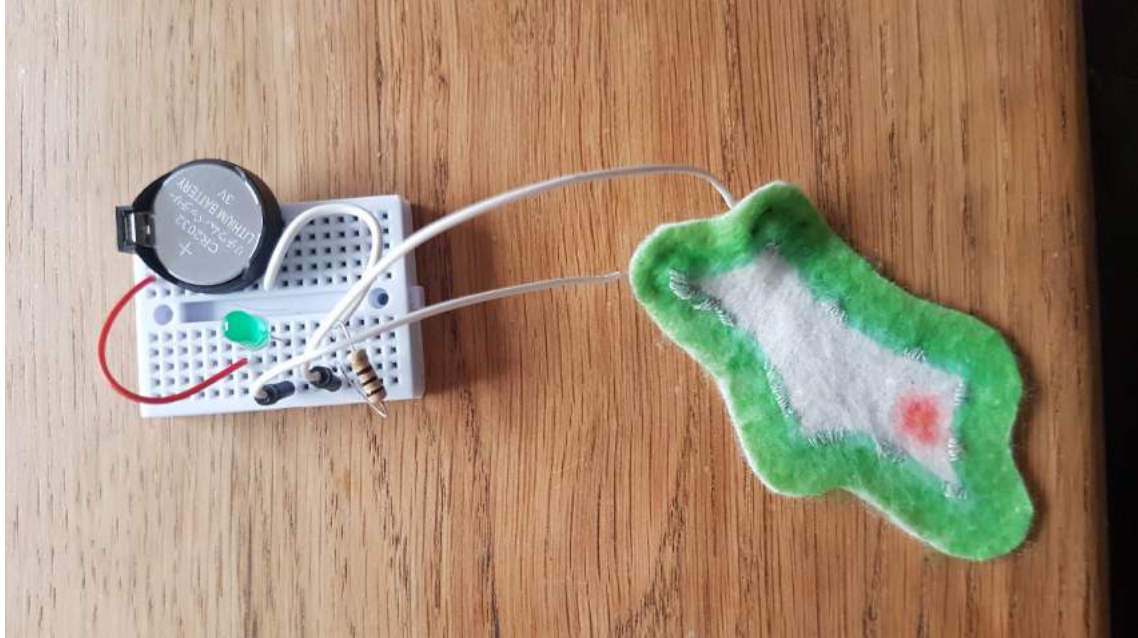
Figure 71: Simple wearable technology kit featuring fabric stretch sensor and bread-board components
