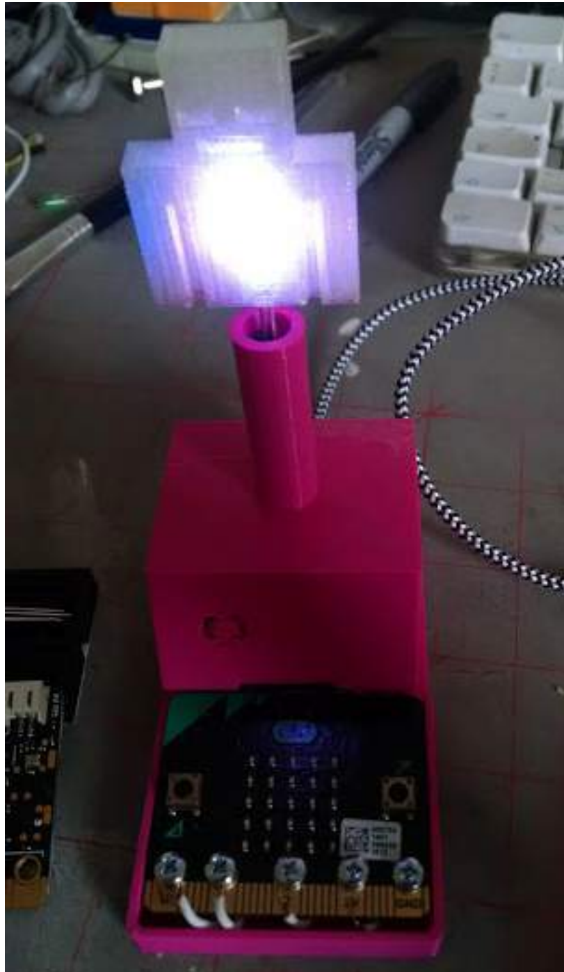
Figure 21: Prototype using microbit and 3D Printed LED Lamp for workshop in 2018 which led to the development of The 3D Print Club at the Neuromuscular Centre
